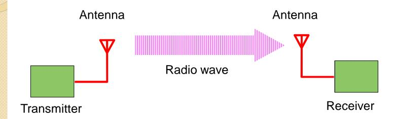
Antennas: important elements of any radio link
